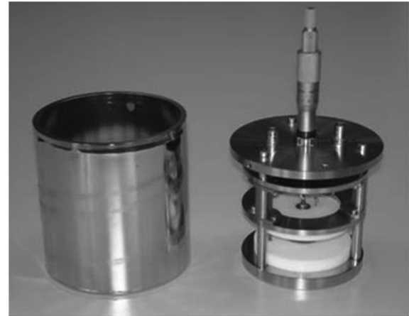
Fig. 1. Dielectric measurement cell described in detail in Ref. [26].
